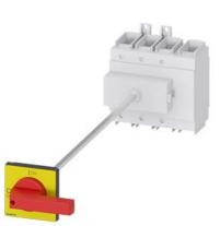
SENTRON, Switch disconnector 3LD, emergency switching-off switch, 4- pole, lu: 160 A, operating power / at AC-23 A 400 V: 75 kW, floor mounting with door coupling, knob-operated mechanism, red/yellow, 4-hole mounting of the handle
