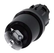
Key-operated switch IKON, 22 mm, round, plastic, lock number 360012K1, with 2 keys, 2 switch positions O-I, latching, actuating angle 90°, 10:30h/13:30h, Key removal O+I
