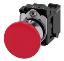
Mushroom pushbutton, 22 mm, round, metal, shiny, red, 40mm, latching, pull-to-unlatch mechanism, with holder, 1 NC, spring-type terminal, with laser labeling, symbol number according to, ISO 7000 or IEC 60417
