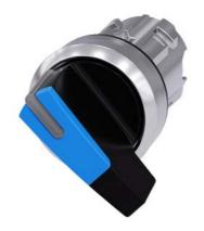
Selector switch, illuminable, 22 mm, round, metal, shiny, blue, selector switch, long, 2 switch positions O<I, momentary contact type, Actuating angle 45°, 10:30h/12h, Z=50-unit packaging
