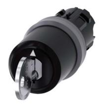
Key-operated switch IKON, 22 mm, round, plastic with metal front ring, lock number 360012K1, with 2 keys, 3 switch positions I>O<II, momentary contact type, actuating angle 2x45°, 10:30h/12h/13:30h, key removal O, with laser labeling, upper case and lower case, always upper case at the beginning of the word
