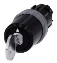
key-operated switch Siemens, 22 mm, round, plastic with metal front ring, lock number SSG10, with 2 keys, 3 switch positions I-O-II, latching, actuating angle 2x45°, 10:30h/12h/13:30h, key removal I+O+II, Z=50-unit packaging
