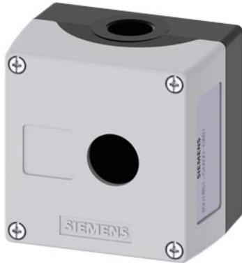
Enclosure for command devices, 22 mm, round, Enclosure material metal, enclosure top part grey, 1 control point, without equipment, Recess for labels, floor mounting, 1xM20 each on top and bottom
