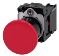
Mushroom pushbutton, 22 mm, round, plastic, red, 40mm, latching, pull-to-unlatch mechanism, with holder, 1 NC, screw terminal, with laser labeling, lower case
