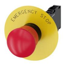
EMERGENCY STOP mushroom pushbutton, 22 mm, round, plastic, red, 40 mm, positive latching, acc. to EN ISO 13850, rotate-to-unlatch, with yellow backing plate, inscription: EMERGENCY STOP, with holder, 1 NO+1 NC, screw terminal, Z=20-unit packaging
