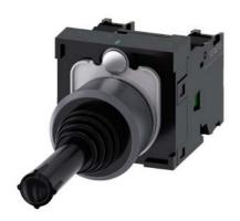
Coordinate switch, 22 mm, round, plastic with metal front ring, black, 2 switch positions, vertical latching, without mechanical interlocking, in O position, with holder, 1 NO, 1 NO, screw terminal, with laser labeling, inscription or symbol, Customer-specific selection with SIRIUS ACT configurator (CIN)
