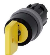
Key-operated switch O.M.R, 22 mm, round, plastic with metal front ring, lock number 73033, yellow, with 2 keys, 3 switch positions I-O-II, latching, actuating angle 2x45°, 10:30h/12h/13:30h, Key removal I+O+II, with laser labeling, upper case
