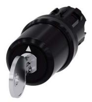
key-operated switch Siemens, 22 mm, round, plastic, special lock, with 2 keys, 3 switch positions I-O<II, left latching, momentary contact type on the right, actuating angle  $2x45^{\circ}$ , 10:30h/12h/13:30h, key removal O
