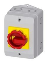
SENTRON, Switch disconnector 3LD, emergency switching-off switch, 3- pole, lu: 25 A, operating power / at AC-23 A 400 V: 9.5 kW, Molded plastic encapsulation for inch cable gland, rotary operating mechanism, red/yellow
