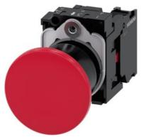
Mushroom pushbutton, 22 mm, round, plastic, red, 40mm, latching, pull-to-unlatch mechanism, with holder, 1 NC, screw terminal, with laser labeling, upper case and lower case, always upper case at the beginning of the word
