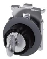
RONIS key-operated switch, 30 mm, round, Metal, matte, front ring for flush installation, special lock, with 2 keys, 3 switch positions I-O-II, latching, actuating angle 2x45°, 10:30h/12h/13:30h, Key removal I+O+II, possible special locks: SB31, 421.455
