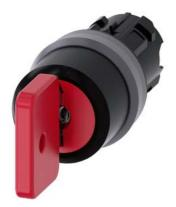
Key-operated switch O.M.R, 22 mm, round, plastic with metal front ring, lock number 73037, red, with 2 keys, 3 switch positions I-O-II, latching, actuating angle 2x45°, 10:30h/12h/13:30h, key removal O, with laser labeling, lower case
