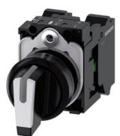
Selector switch, illuminable, 22 mm, round, plastic, white, selector switch, short, 3 switch positions I-O-II, latching, 10:30h/12h/13:30h, with holder, 1 NO, 1 NO, spring-type terminal, Z=20-unit packaging
