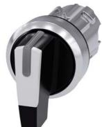
Selector switch, illuminable, 22 mm, round, metal, shiny, white, selector switch, long, 3 switch positions I-O-II, latching, actuating angle 2x45°, 10:30h/12h/13:30h
