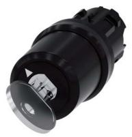
Key-operated switch BKS, 22 mm, round, plastic, lock number S1, with 2 keys, 2 switch positions O-I, latching, actuating angle  $90^\circ$ , 10:30h/13:30h, Key removal O+I
