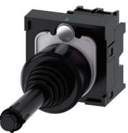
Coordinate switch, 22 mm, round, plastic, black, 2 switch positions, vertical, momentary contact type, with mechanical interlocking in O position, with holder, 1 NO, 1 NO, screw terminal
