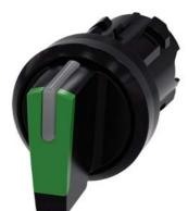
Selector switch, illuminable, 22 mm, round, plastic, green, selector switch, short, 3 switch positions |>O<II|, momentary contact on the left, latching on the right, actuating angle 2x45°, 10:30h/12h/13:30h, with laser labeling, upper case and lower case, always upper case at the beginning of the word
