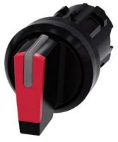
Selector switch, illuminable, 22 mm, round, plastic, red, selector switch, short, 3 switch positions I>O<II, momentary contact type, actuating angle  $2x45^{\circ}$ , 10:30h/12h/13:30h, with laser labeling, upper case and lower case, always upper case at the beginning of the word
