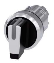
Selector switch, illuminable, 22 mm, round, metal, shiny, white, selector switch, short, 3 switch positions I-O<II, left latching, right momentary contact type, actuating angle  $2x45^{\circ}$ , 10:30h/12h/13:30h, Z=50-unit packaging
