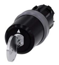
Key-operated switch BKS, 22 mm, round, plastic with metal front ring, lock No. E9 (VW), without key, 3 switch positions I-O-II, latching, actuating angle  $2x45^{\circ}$ , 10:30h/12h/13:30h, Key removal I+O+II, with laser labeling, lower case
