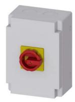
SENTRON, Switch disconnector 3LD, emergency switching-off switch, 3- pole, lu: 125 A, operating power / at AC-23 A 400 V: 45 kW, Molded plastic encapsulation for inch cable gland, rotary operating mechanism, red/yellow
