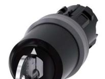
Key-operated switch IKON, 22 mm, round, plastic with metal front ring, lock number 360012K1, with 2 keys, 3 switch positions I-O<II, left latching, right momentary contact type, actuating angle 2x45°, 10:30h/12h/13:30h, Key removal O+I
