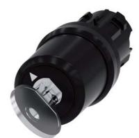
Key-operated switch BKS, 22 mm, round, plastic, lock No. E9 (VW), without key, 2 switch positions O-I, latching, actuating angle 90°, 10:30h/13:30h, key removal O, with laser labeling, inscription or symbol Customer-specific selection with SIRIUS ACT configurator (CIN)
