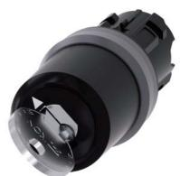
Key-operated switch IKON, 22 mm, round, plastic with metal front ring, lock number 360012K1, with 2 keys, 2 switch positions O-I, latching, actuating angle 90°, 10:30h/13:30h, key removal O, with laser labeling, lower case
