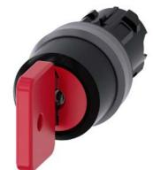
Key-operated switch O.M.R, 22 mm, round, plastic with metal front ring, lock number 73037, red, with 2 keys, 3 switch positions I>O<II, momentary contact type, actuating angle 2x45°, 10:30h/12h/13:30h, key removal O, with laser labeling, upper case
