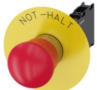
EMERGENCY STOP mushroom-type actuator, 22 mm, round, metal, shiny, red, 40 mm, positive latching, according to EN ISO 13850, rotate-to-unlatch, with yellow backing plate, inscription: NOT-HALT, with holder, 1 NO+1 NC, spring-type terminal
