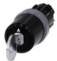
key-operated switch Siemens, 22 mm, round, plastic with metal front ring, lock number SSG10, with 2 keys, 3 switch positions I-O<II, left latching, momentary contact type on the right, actuating angle  $2x45^{\circ}$ , 10:30h/12h/13:30h, key removal O+I, with laser labeling, upper case and lower case, always upper case at beginning of line
