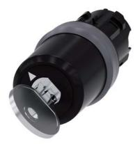
Key-operated switch BKS, 22 mm, round, plastic with metal front ring, lock number S1, with 2 keys, 2 switch positions O-I, latching, actuating angle  $90^\circ$ , 10:30h/13:30h, Key removal I
