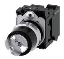
RONIS key-operated switches, 22 mm, round, metal, shiny, lock number SB30, with 2 keys, 2 switch positions O-I, latching, 90° operating angle, 10:30/1:30 o'clock, key removal O+I, with holder, 1NO, spring-type terminals, possible special locks: SB31, 421, 455, Z=20-unit packaging
