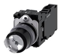
RONIS key-operated switch, 22 mm, round, plastic with metal front ring, lock number SB30, with 2 keys, 2 switch positions O-I, latching, actuating angle 90°, 10:30h/13:30h, key removal O+I, with holder, 1 NO+1 NC, screw terminal, possible special locks: SB31, 421, 455, with laser labeling, lower case
