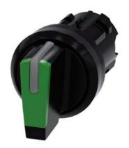
Selector switch, illuminable, 22 mm, round, plastic, green, selector switch, short, 3 switch positions I-O<II, left latching, right momentary contact type, actuating angle 2x45°, 10:30h/12h/13:30h, with laser labeling, inscription or symbol Customer-specific selection with SIRIUS ACT configurator (CIN)
