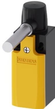
Hinge switch Plastic enclosure, 31 mm according to EN 50047 Device connection 1 x (M20 x 1.5) 1 NO/1 NC quick action contacts integrated, with solid shaft Diameter = 10 mm Actuating angle 10°
