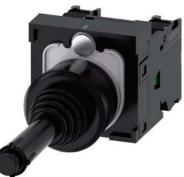
Coordinate switch, 22 mm, round, plastic, black, 2 switch positions, horizontal latching, with mechanical interlocking, in O position, with holder, 1 NO, 1 NO, screw terminal, with laser labeling, lower case
