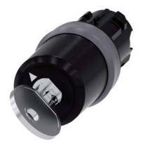
key-operated switch Siemens, 22 mm, round, plastic with metal front ring, lock no. LSG1, with 2 keys, 2 switch positions O-I, latching, actuating angle 90°, 10:30h/13:30h, key removal O, with laser labeling, upper case and lower case, always upper case at beginning of line
