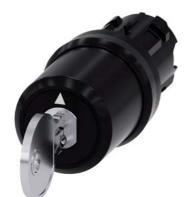
keyswitch BKS, 22 mm, round, plastic, special lock, with 2 keys, 3 switch positions I-O-II, latching, actuating angle 2x45°, 10:30h/12h/13:30h, key removal I, note: for the BKS locking systems E1 - E25 supplied without key
