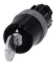
Key-operated switch BKS, 22 mm, round, plastic with metal front ring, lock number S1, with 2 keys, 3 switch positions I>O<II, momentary contact type, actuating angle  $2x45^{\circ}$ , 10:30h/12h/13:30h, Key removal O
