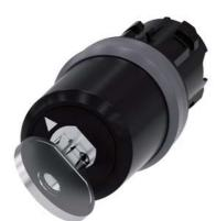
Key-operated switch BKS, 22 mm, round, plastic with metal front ring, lock number S1, with 2 keys, 2 switch positions O-I, latching, actuating angle 90°, 10:30h/13:30h, key removal O+I, Z=50-unit packaging
