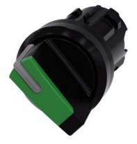
Selector switch, illuminable, 22 mm, round, plastic, green, selector switch, short, 2 switch positions O<I, momentary contact type, Actuating angle 45°, 10:30h/12h, with laser labeling, upper case
