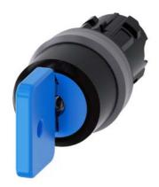
Key-operated switch O.M.R, 22 mm, round, plastic with metal front ring, lock number 73038, blue, with 2 keys, 3 switch positions I-O-II, latching, actuating angle 2x45°, 10:30h/12h/13:30h, Key removal I+O+II, with laser labeling, inscription or symbol Customer-specific selection with SIRIUS ACT configurator (CIN)
