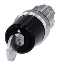
Key-operated switch BKS, 22 mm, round, metal, shiny, lock number S1, with 2 keys, 3 switch positions I-O-II, latching, actuating angle 2x45°, 10:30h/12h/13:30h, Key removal I+II, with laser labeling, upper case and lower case, always upper case at the beginning of the word
