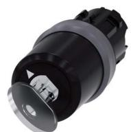
Key-operated switch BKS, 22 mm, round, plastic with metal front ring, lock number S1, with 2 keys, 2 switch positions O-I, latching, actuating angle 90°, 10:30h/13:30h, key removal I, with laser labeling, upper case and lower case, always upper case at beginning of line
