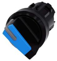
Selector switch, illuminable, 22 mm, round, plastic, blue, selector switch, short, 2 switch positions O-I, latching, actuating angle  $90^\circ$ , 10:30h/13:30h, with laser labeling, upper case and lower case, always upper case at the beginning of the word
