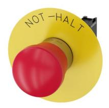
EMERGENCY STOP mushroom pushbutton, 22 mm, round, metal, shiny, red, 40 mm, positive latching, according to DIN EN ISO 13850, pull to unlatch, with yellow backing plate, inscription: NOT-HALT, with holder, 1 NC, screw terminal, Z=20-unit packaging
