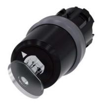
Key-operated switch BKS, 22 mm, round, plastic with metal front ring, Lock No. E9 (VW), without key, 2 switch positions O-I, latching, actuating angle  $90^\circ,\,10:\!30h/13:\!30h,$  Key removal O
