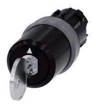
Key-operated switch BKS, 22 mm, round, plastic with metal front ring, lock number S1, with 2 keys, 3 switch positions I-O-II, latching, actuating angle  $2x45^{\circ}$ , 10:30h/12h/13:30h, key removal O, Z=50-unit packaging
