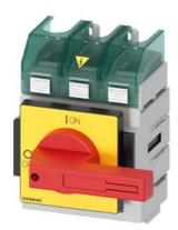
SENTRON, Molded case switch 3LD5 UL, Emergency switching-off, 3-pole, certified according to UL489 UL60947-4-1 and IEC60947-3, UL: 100A, SCCR 65kA at 480VAC, Operating power at 480VAC 3-phase: 60hp, IEC: 100A, Operating power at AC-23A at 400V: 45kW, floor mounting with direct handle, red/yellow, incl. terminal covers for the infeed side
